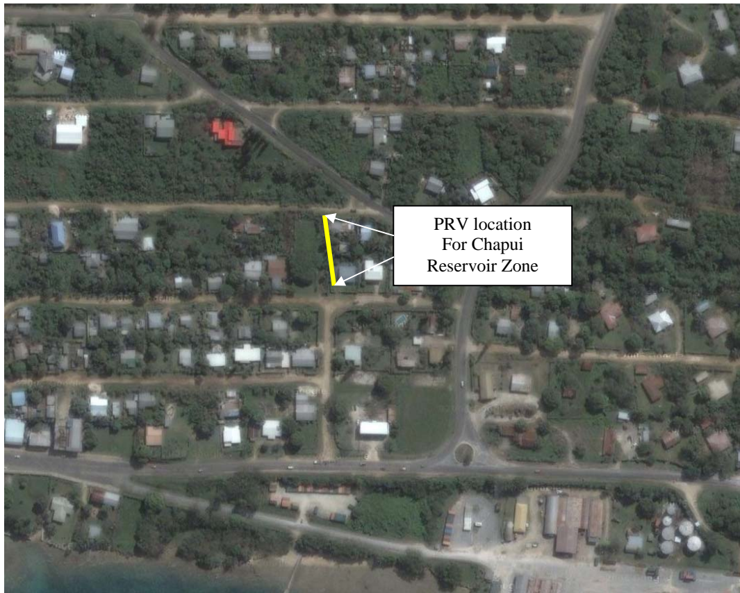
Possible location of PRV for the proposed Chapui Pressure management Zone (part of the proposed Chapui District Metered Area).
